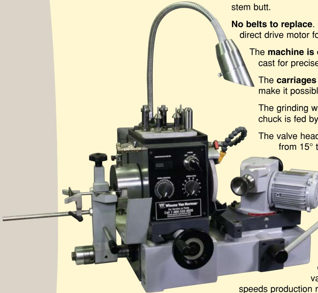
The VRX Valve Refacing/Grinder machine will reface the valve and also chamfer/recondition the valve stem butt.
