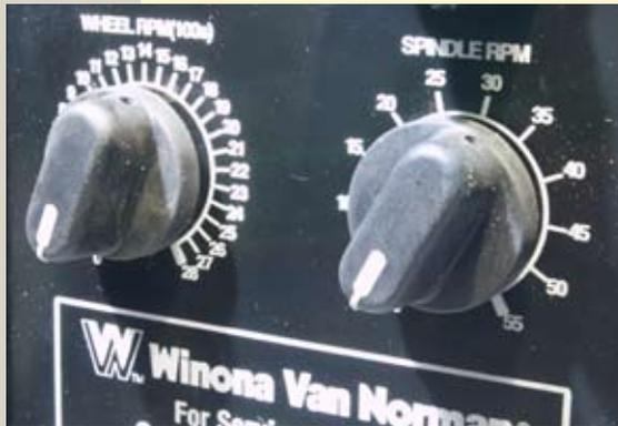
Variable speeds for different valve diameters and surface finishes.
