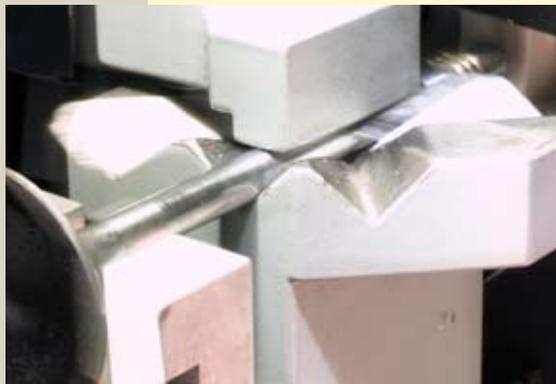
V-ways and clamping system for accurate valve stem butt end grinding and chamfering.
